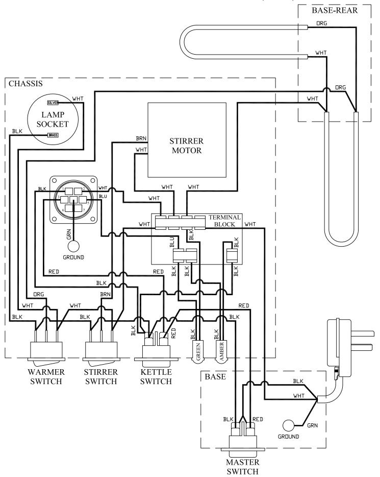
TP-16 & 20 WIRING DIAGRAM (230V)
