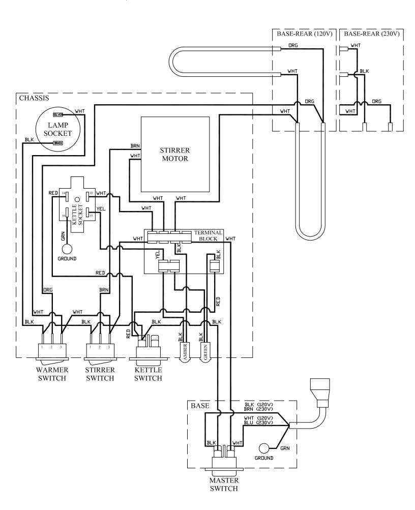
PS/TP-16 WIRING DIAGRAM (120V)
